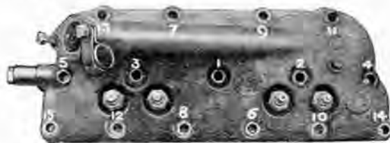
The order in which the cylinder head holding down nuts should be loosened and tightened up.
