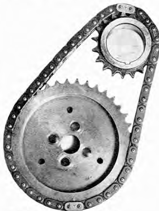
Here is shown the correct position for the sprockets and chain to ensure correct timing.
