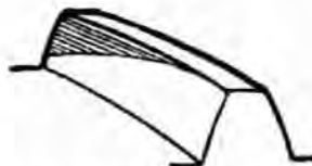
Fig. 5. This marking is incorrect and is caused by the pinion being too far into mesh with the crown wheel. To correct, adjust pinion away from crown wheel and reset backlash.
