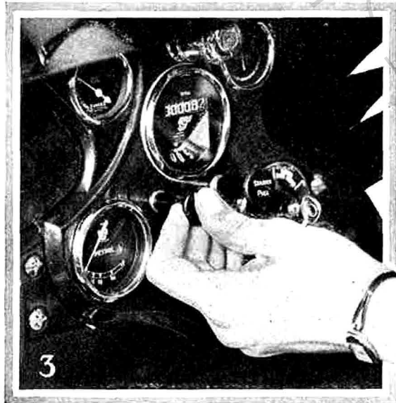
3.—Then push the mixture control back towards the dash as far as it will go, and allow the engine to run until normal working temperature is attained.
