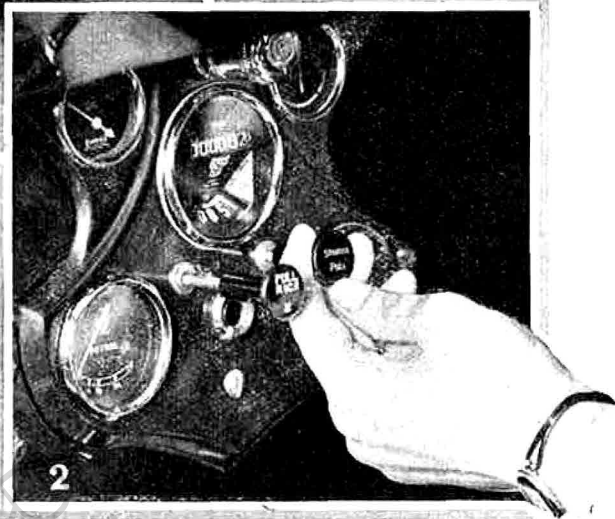
2.—Start the engine (with the mixture control pulled out) by pulling the starter knob.
