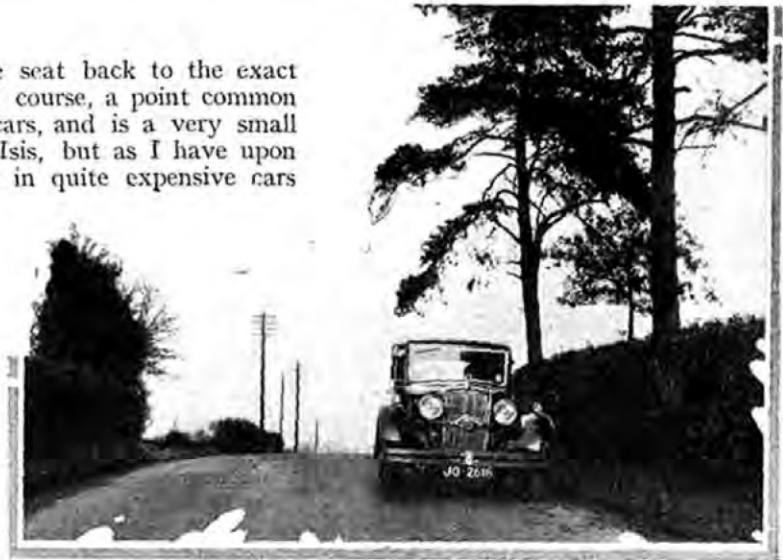
This frontal view gives an idea of the attractiveness of the new radiator, which has chromium finished shutters automatically operated.
