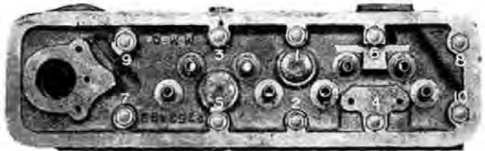
The correct order in which the cylinder head stud nuts should be gradually slackened or tightened is here indicated.
