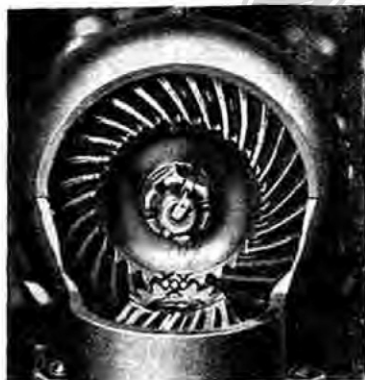
(Left) The timing marks on the camshaft bevel wheels. The marked tooth of the driving pinion should engage between the marked teeth of the camshaft bevel.
