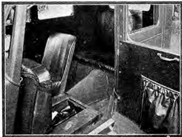
The front seats tip forward and the backs fold over, affording easy access to the rear seats. Note the well for the rear passengers' feet and the handy toolbox.
