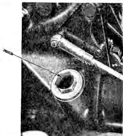
FIG. 45. THE GEARBOX FILLING ORIFICE AND LEVEL INDICATOR
