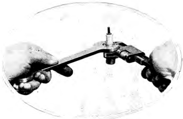
FIG. 24. TAKING A PLUG TO PIECES FOR CLEANING PURPOSES
