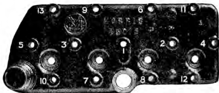
FIG. 20. SHOWING THE SEQUENCE IN WHICH THE CYLINDER HEAD STUD NUTS SHOULD BE TIGHTENED
