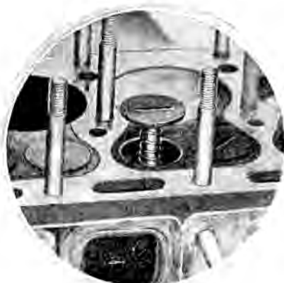
FIG. 16. SHOWING USE OF SPRING TO FACILITATE VALVE GRINDING
