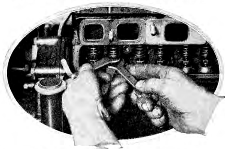
FIG. 18. TIGHTENING UP THE TAPPETS AFTER ADJUSTMENT
