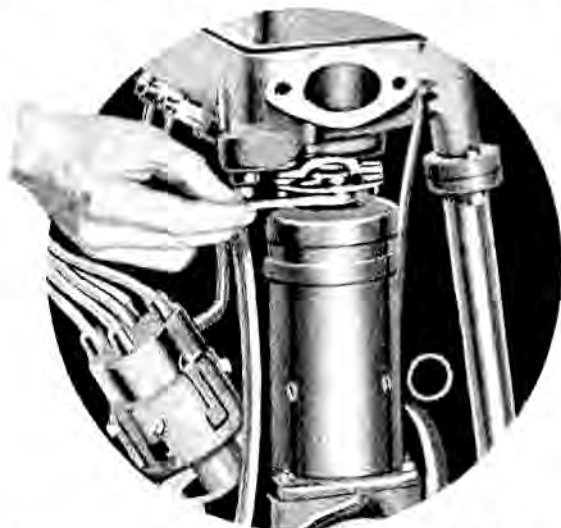
FIG. 62. REMOVING THE COUPLING BOLTS OF THE FLEXIBLE COUPLING
