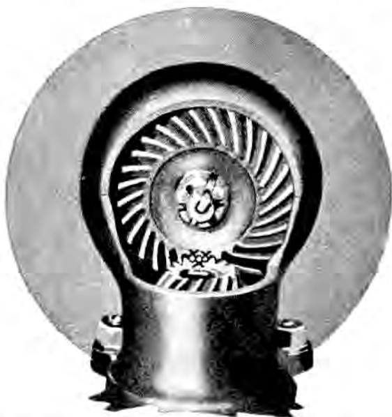
FIG. 59. THE CAMSHAFT TIMING WHEEL. MARKS CAN BE CLEARLY SEEN
