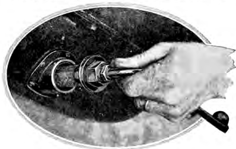
FIG. 44. REMOVING OIL FILTER FROM SUMP FOR CLEANING PURPOSES
