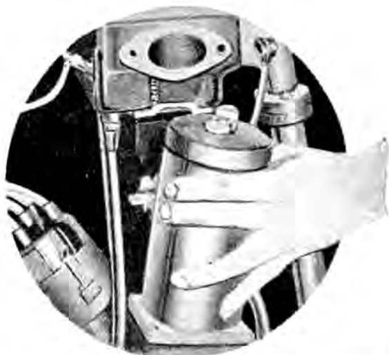
FIG. 63. SHOWING HOW THE DYNAMO SHOULD BE REMOVED OR REPLACED
