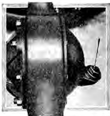
FIG. 46. REAR AXLE FILLING ORIFICE AND LEVEL-INDICATOR
