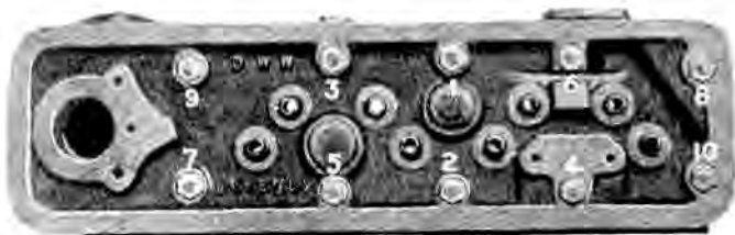
FIG. 61. SEQUENCE OF TIGHTENING CYLINDER-HEAD STUD NUTS
