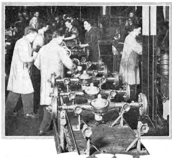
The end of the axle assembly line, showing finished axles undergoing final inspection before being transferred to the spray painting booth.
