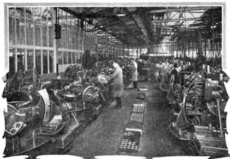
The battery of special machines used to cut the spiral bevel gears used on the Morris Minor.
