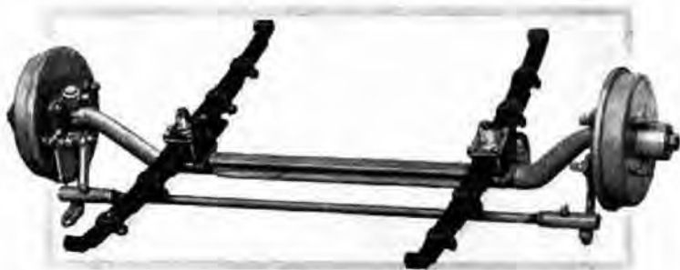
The front axle assembly of the Morris Minor.
