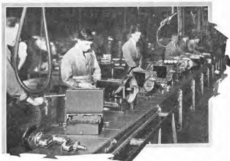
A portion of the Morris Minor engine assembly conveyor on which the engines are assembled.
