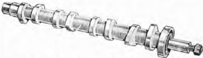
The camshaft is of generous dimensions and carried on ball and roller bearings.
