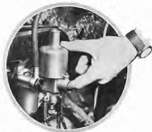
By inserting a finger in the air intake the piston may be raised or lowered to free its action.
