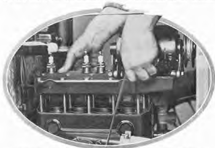
The cylinder head can easily be lifted from the studs in the manner indicated or by standing on the bonnet boards astride the engine.
