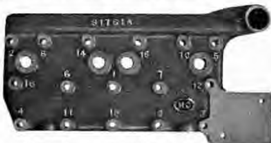
Indicating the sequence in which the cylinder head stud nuts should gradually be tightened.
