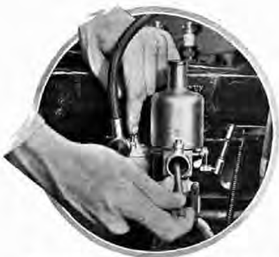
To observe the petrol flow from the jet, the piston should be raised with a small implement and the float-chamber flooded by raising the protruding needle.
