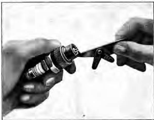
Adjustments should be made only by the side wire, and the combined setting tool and gap gauge illustrated can be obtained from the Champion Sparking Plug Co. or your Morris Dealer for 4d.
