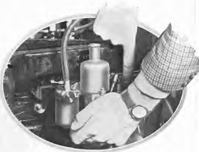
An obstructed jet should be cleared by opening the throttle by means of the accelerator rod while the engine is running and momentarily closing the air intake with the other hand.
