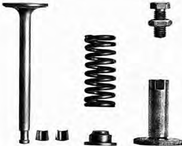
The component parts of the valve and valve tappet, consisting of the valve, valve cotters, valve spring, valve spring cap, tappet screw and lock nut, and the tappet.
