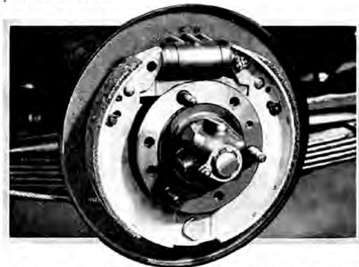
The brake-drum removed, showing the rear brake-shoe assembly. The assembly for the front shoes is identical, with the exception of the hand-operating mechanism.
