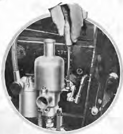
Adjusting the carburetter throttle stop screw to obtain the correct slow-running position after setting the jet.
