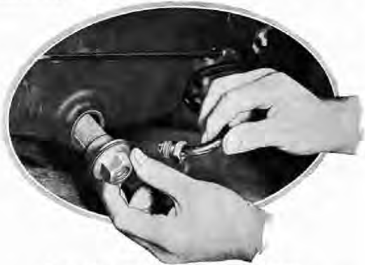
How the oil filter is withdrawn from the sump for cleaning purposes.
