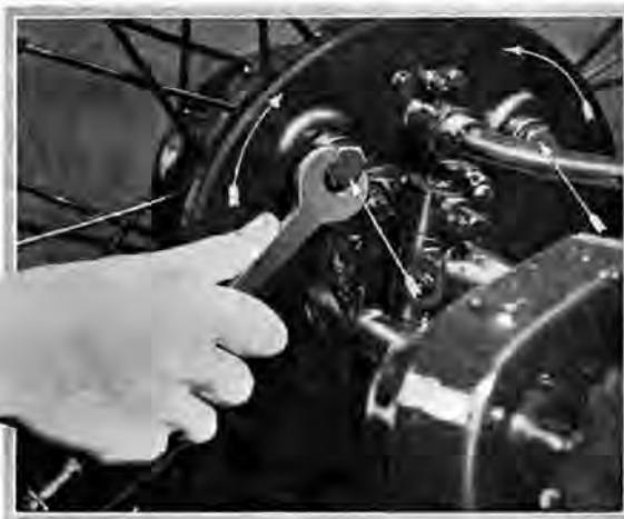
Here are shown the brake adjusting bolts, which when rotated away from the centre of the wheel bring the shoes closer to the drum, and when rotated in the direction shown by the arrows bring the shoes farther from the drum.
