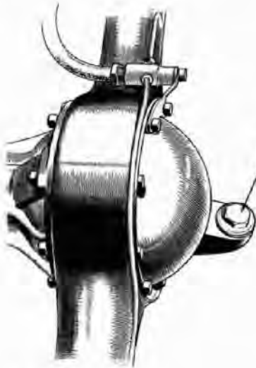
The oil filling plug of the Morris Minor rear axle, which also serves to regulate the oil level.
