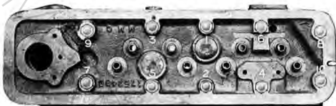
Indicating the sequence in which the cylinder head stud nuts should gradually be tightened.
