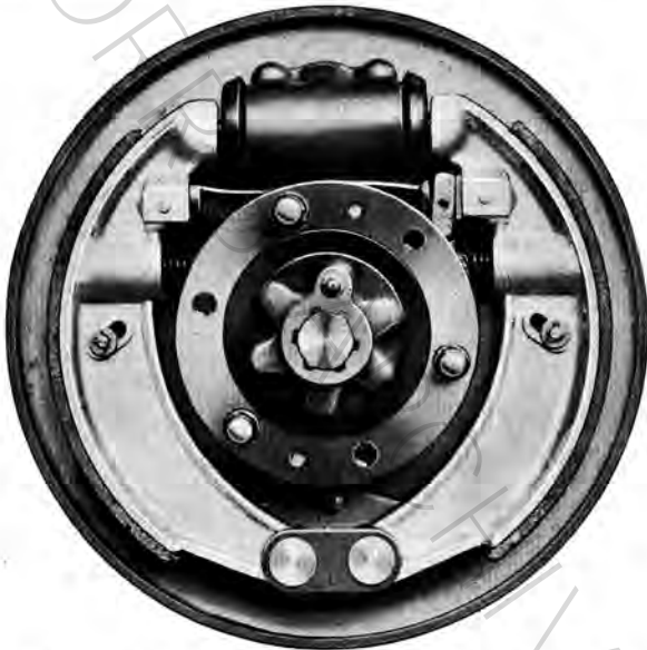
The Morris Eight brake-drum removed, showing the rear brake-shoe assembly. The assembly for the front shoes is identical, with the exception of the hand-operating mechanism.
