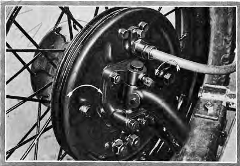
Indicating the brake-shoe adjusting nuts. These should be rotated in the direction indicated by the small arrows to bring the shoes farther away from the drum and in the opposite direction to bring the shoes closer to the drum.
