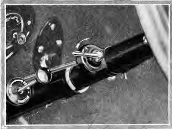
The ignition control on the steering column of the Morris Family Eight. The arrow indicates the direction of motion for advancing the ignition.
