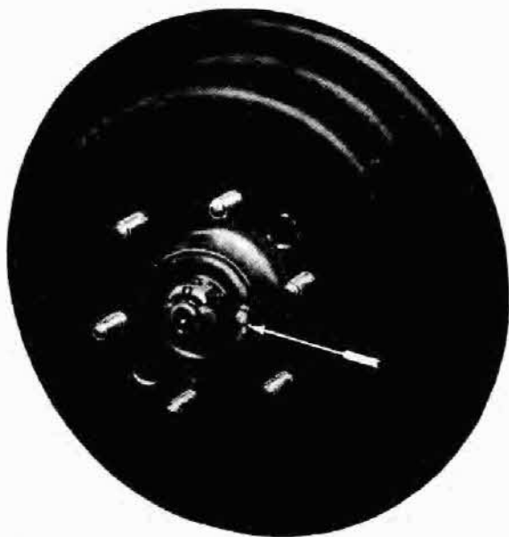
The front hub oil nipples can clearly be seen just beside the hub nut.
