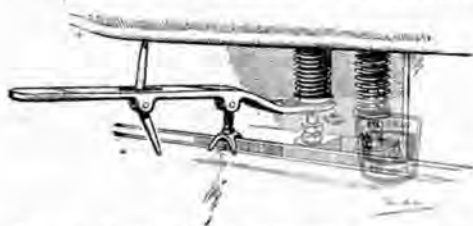
Fig. 2.—A special tool makes the removal or replacement of a valve spring an easy matter.
