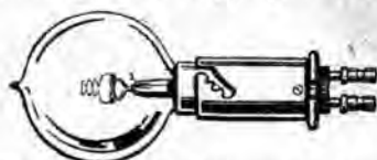
Fig. 5.—Three notches are provided in the bulb holder to allow for focussing.
