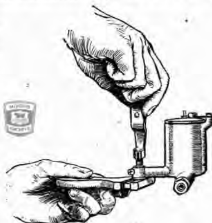
Fig. 5.—How the jet may be detached by means of the special spanner provided.
