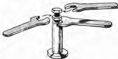
Fig. 3.—Three small spanners are provided for tappet adjustment and are used as shown.
