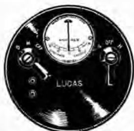
Fig. 3.—Two switches and an ammeter are contained in the switchbox.
