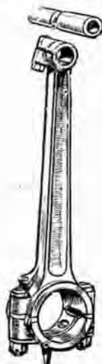
Fig. 5.—Connecting rod and gudgeon pin of the 1924 Cowley engine. Shims are fitted in the big-end bearings to provide an easy means of taking up wear.
