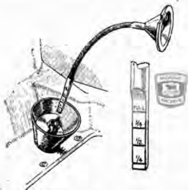
Fig. 8.—Oil filler orifice on the crank case, and oil level indicator.
