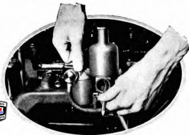
To observe the petrol flow from the jet, the piston should be raised with a small implement and the float-chamber flooded by raising the protruding needle.
