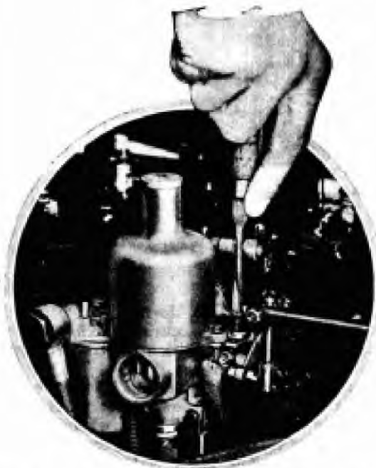
Adjusting the carburettor throttle stop screw to obtain the correct slow-running position after setting the jet.
