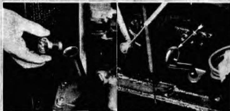
The oil filler and graduated dipper rod on the Morris Eight.
