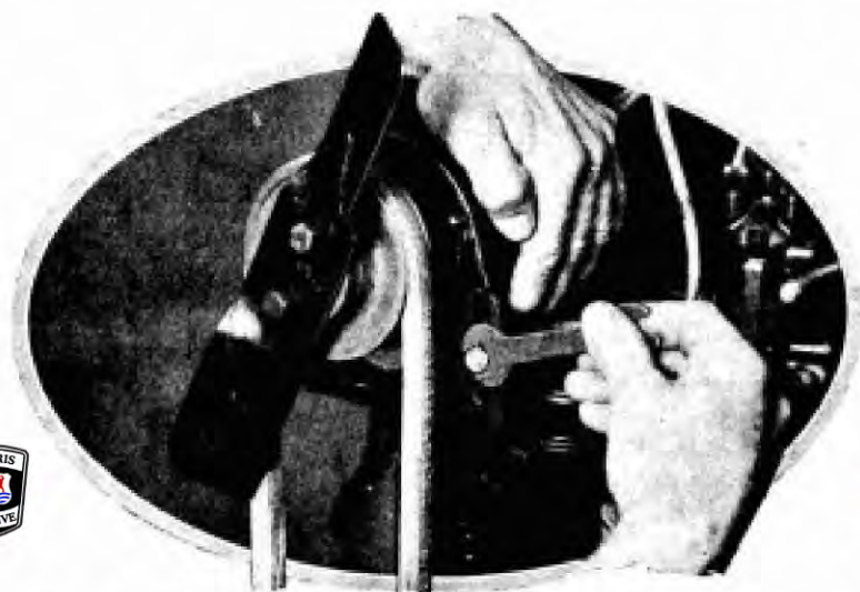
The fan belt tension is adjusted by slackening the dynamo fixing nuts while supporting the dynamo with the other hand.
