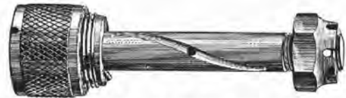
Combination Shackle Bolt and Lubricator as fitted to De Luxe Models.
