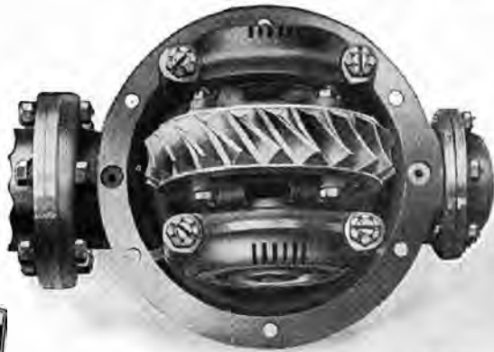
Back Axle Worm Gear. Differential dismantled showing accessibility.
