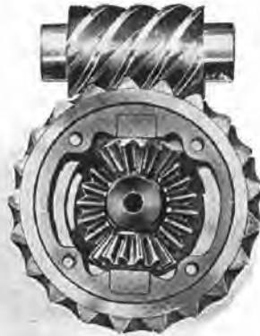
Back Axle Worm Gear. Differential dismantled showing accessibility.
