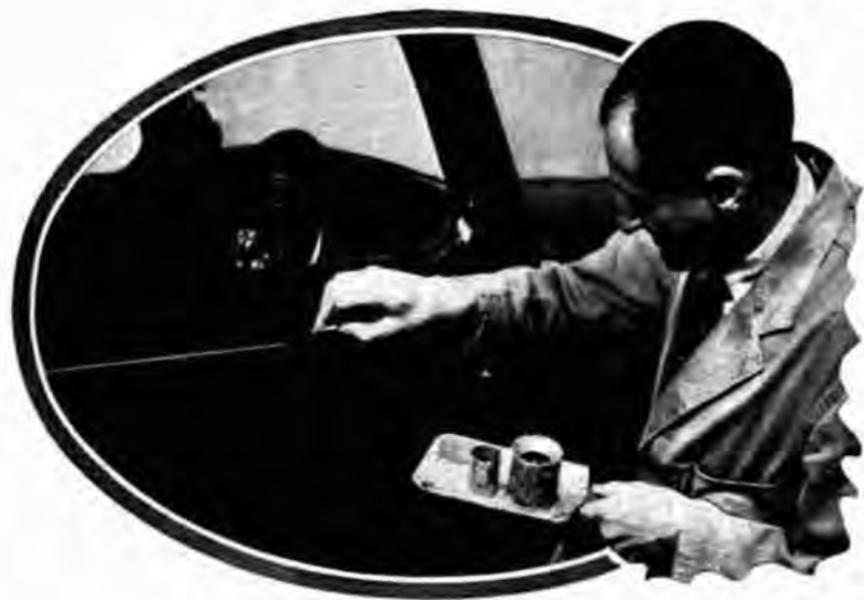
Fig. 6. Left.—If the repair has taken place in the region of the car lining, the obliterated line should be restored carefully.
