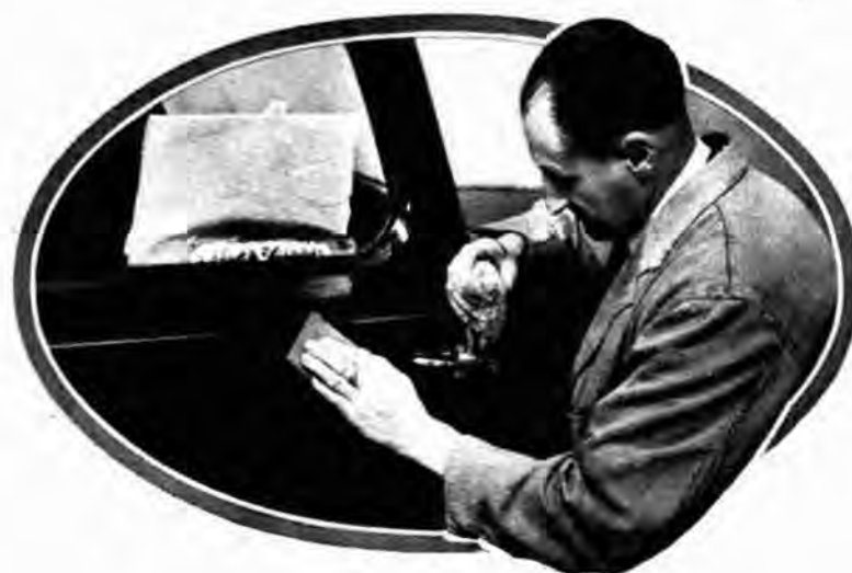
Fig. 4. Left.—When the "Synobel" film has been sufficiently hardened off by the application of the infra-red lamp the surface should be faced carefully with No. 500 "Wet-or-dry" paper.
