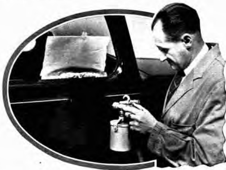
Fig. 3. Right.—Application of the "Synobel" finish with the spray gun, using a No. 90 nozzle with air restrictor adaptor.
