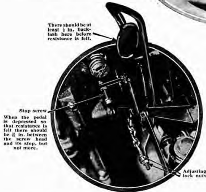
Fig. 3. Left.—The Morris Eight (Series "E") Clutch Setting. The clutch pedal adjustment on the Morris Eight consists of a screwed eyebolt with two locating lock nuts.
