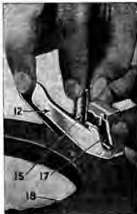
Fig. 6. Above.—The correct method of removing and assembling the clutch release levers can be followed from this illustration.
