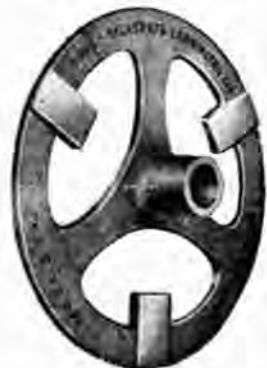
Fig. 8. Below.—The special Borg and Beck gauge plate necessary for setting the release levers.
