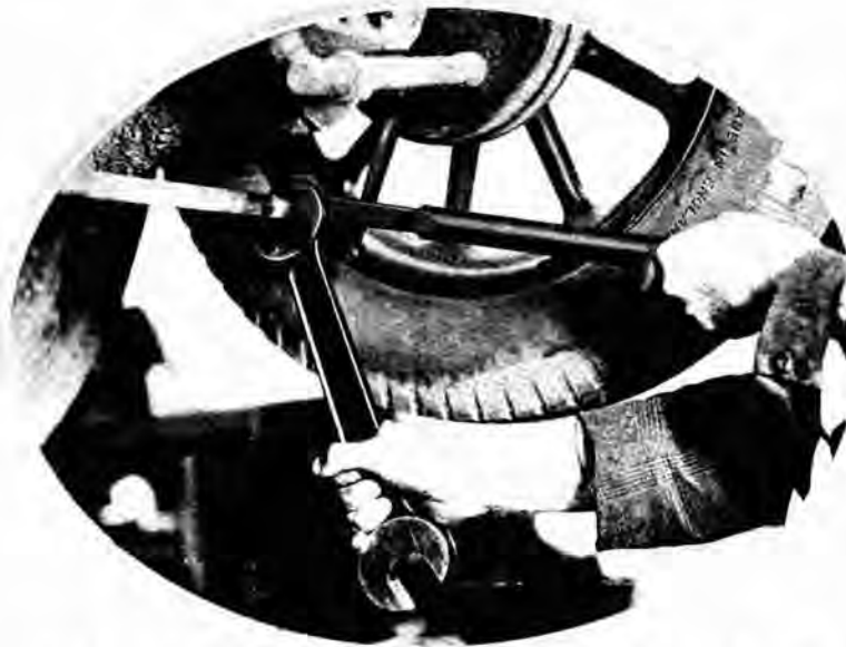
It is essential to hold the ball end socket centrally against rotation with an adequate spanner while tightening or slackening the lock nut.
