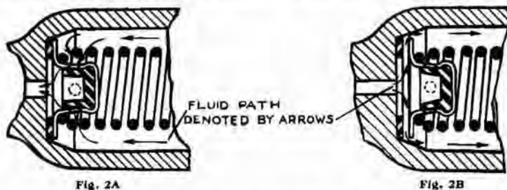
These two figures illustrate the manner in which the outlet check valve functions.
