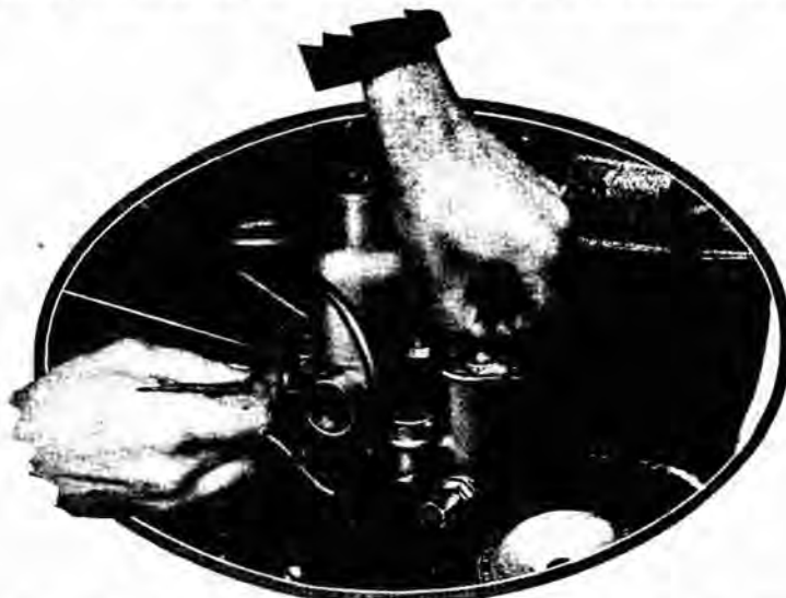
To observe the flow of petrol from the jet, the piston should be raised with a small implement and the float-chamber flooded by raising the protruding needle.
