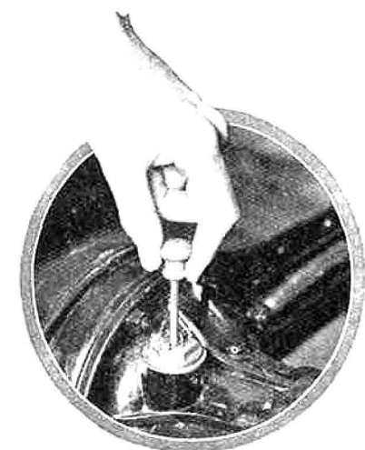
A dipstick is fitted to the rear axle casing on the Morris Eight—
