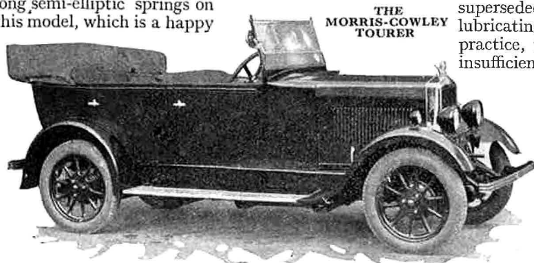
The Morris-Cowley Tourer, which has a modified head to its engine, lighter valves and an even better performance than hitherto.
