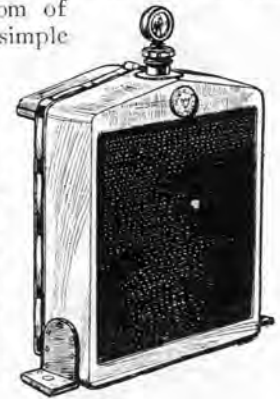
The new flat-fronted radiator.
