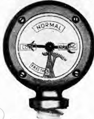
The Calometer, a temperature-recording device which is readable equally as well by night as in the daytime. It is a new fitment on all models.
