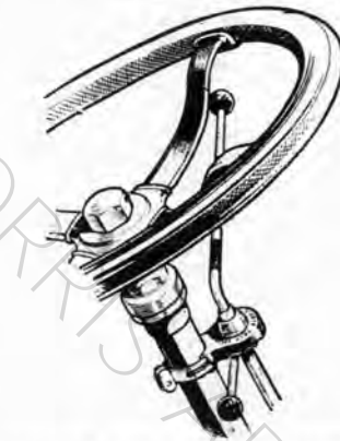
(ABOVE) THE MIXTURE CONTROL ON THE MORRIS-OXFORD. (LEFT) DRAUGHT-EXCLUDING FLAP ON SIDE CURTAINS. (RIGHT) WATER GUTTER ON THE TWO-PANEL SCREENS.
