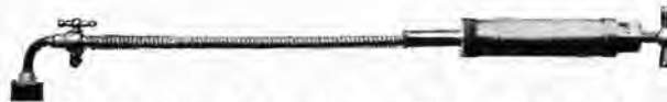
In the equipment is a screw-down oil gun, the union of which fits every oil cup on the car.
