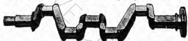
Three-bearing balanced crankshaft of the Morris engine.
