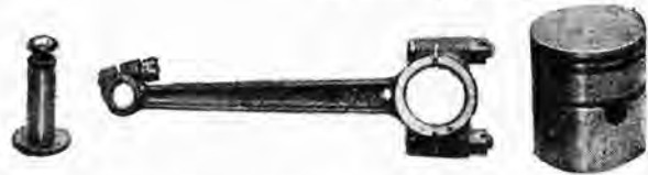
Mushroom ended tappet, connecting rod with cotter gudgeon pin fixing, and three-ringed cast iron piston of the Morris-Oxford engine.
