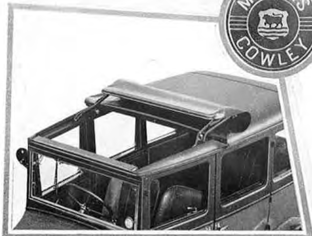
The folding head is easily operated and weatherproof when closed.
