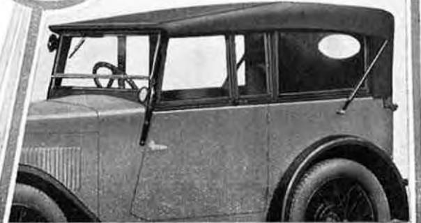
Showing the all-weather equipment in position.
