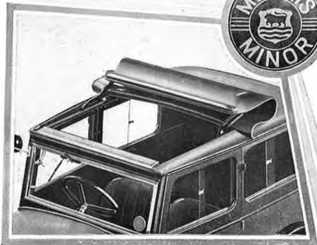
Showing the folding head open. It is very easily and quickly operated, and when down is absolutely weatherproof.
