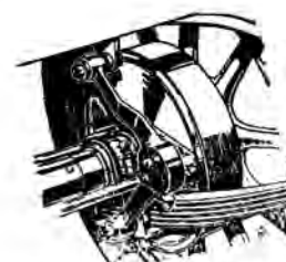
Showing the underslung rear spring and method of attachment of rear shock absorbers
