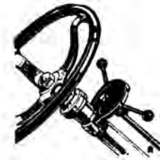
New improved magneto and carburetter controls on steering column
